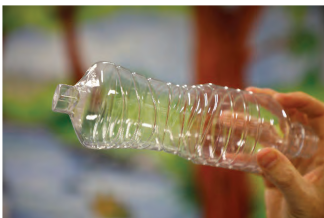
Figure 2: The bottle spacer as produced with the protuberance
