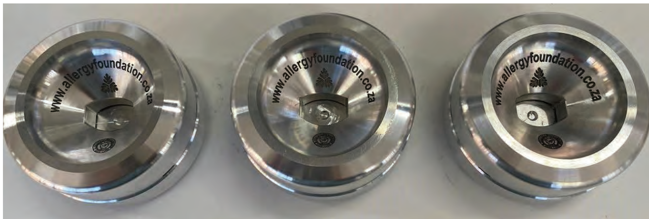
Figure 1: The base for the blow-mould machines
