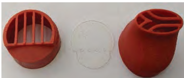
Figure 9: The three components of the AfriValve prototype manufactured using a 3D printer and cast silicone
